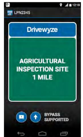
The driver in bypass service will always receive a *Conditional Bypass* at Florida Agriculture sites. Prior to reaching the site entry point, the display will clearly indicate the driving instruction for all vehicles to bypass the Drivewyze supported inspection site on the condition they are not driving **Reefer trucks** or hauling **agriculture, horticulture** or **aquaculture** loads.
